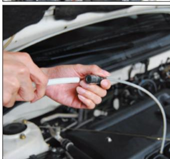
4. After oil extraction, turn the lever to the "CLOSE" position and disconnect the air line from the unit. Remove the extracting tube from the dipstick tube (refit the oil dipstick). Remove the main suction tube from the unit. Slowly pour the used oil into a suitable container and dispose of it in an appropriate manner.
