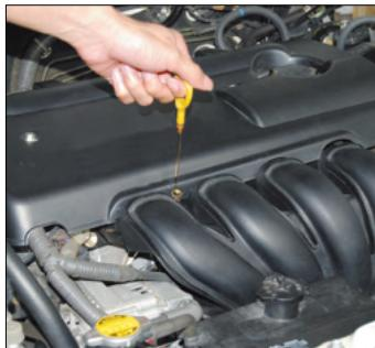
2. Select and insert the appropriate diameter extracting tube into the dipstick until it reaches the bottom of the oil pan, connect the main suction tube to the unit and to the extracting tube.
